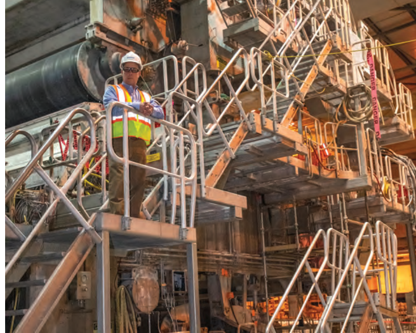
Troy Wilson stands halfway up a hulking machine designed to press the liquid out of the containerboard before sending it on to heated rollers that will dry it out.
